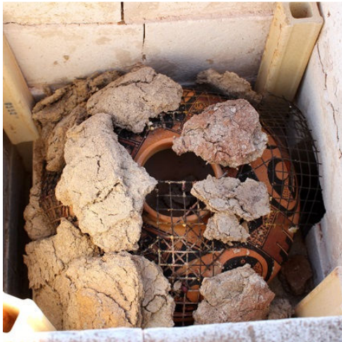
Figure 4(c). Pot with more dung placed around the pot inside kiln after firing.
