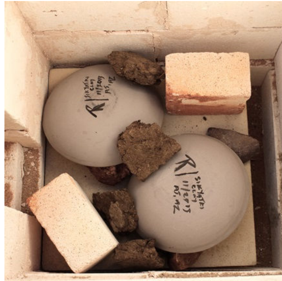
Figure 3(b). The two test bowls in the kiln with pieces of sheep dung, before firing.
