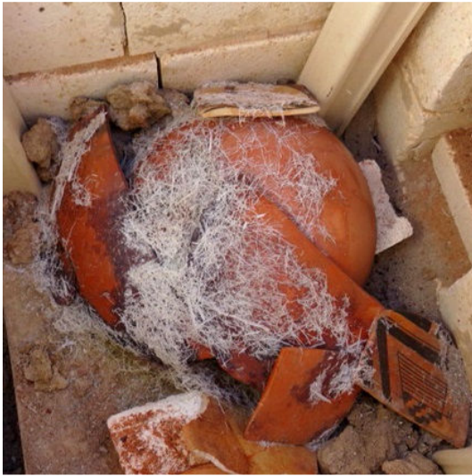
Figure 6(c). Re-fired bowl and sherds inside gas test kiln after firing with salt-soaked straw.
