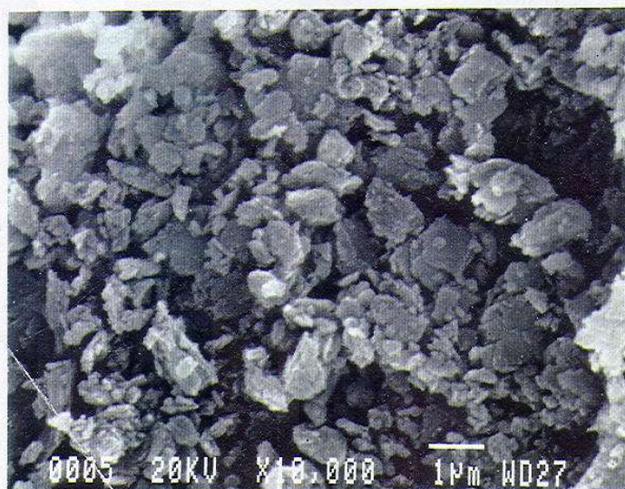
Figure 8. Undeformed clay minerals in the substrate of Sample 5..
