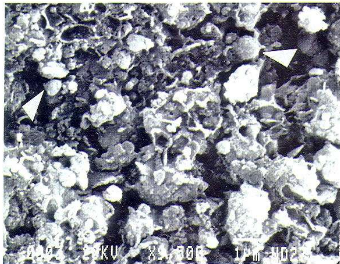
Figure 6. Maghemite particles (arrows) in Sample 5 that retain the form of hematite.
