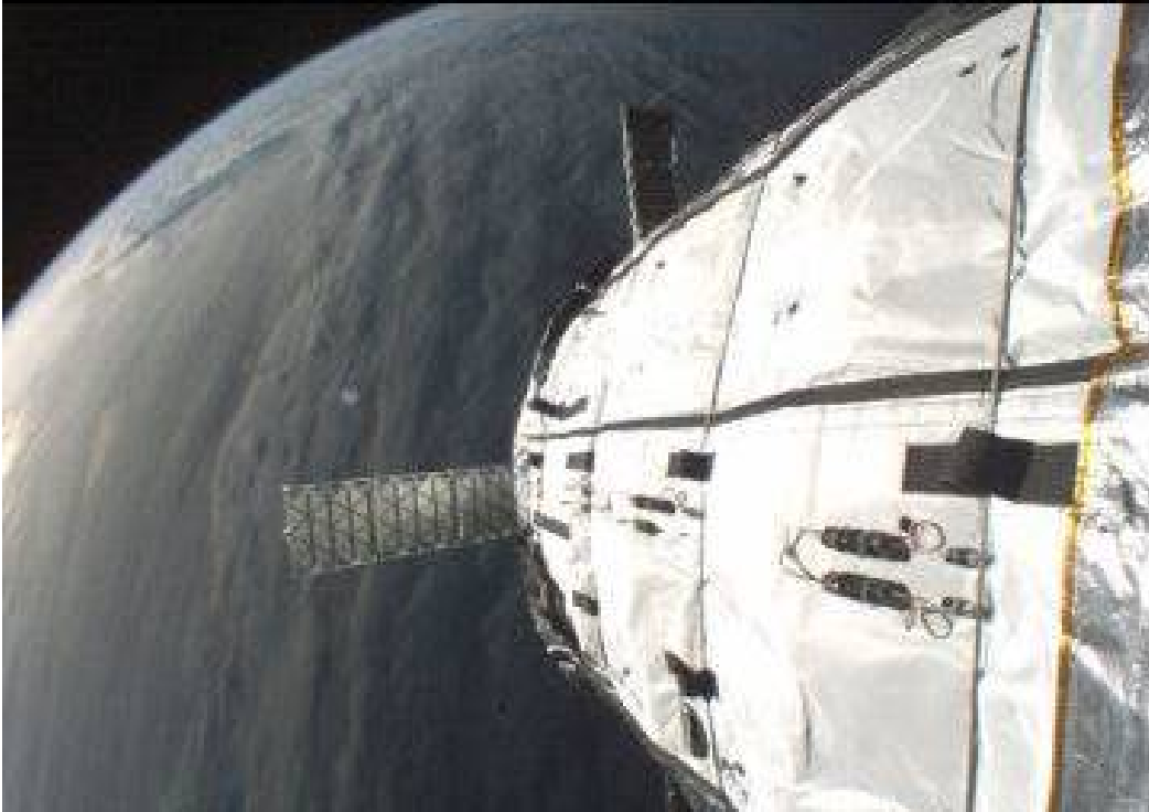
A cloud covered vista of Earth passes below the fully inflated Genesis II spacecraft. Bigelow's designs incorporate inflatable module technology developed by NASA during the TransHab program. (Bigelow Aerospace)
