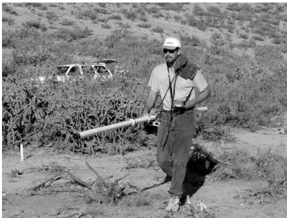
Figure 2 Garth Hayden carries an EM-31 electromagnetic induction instrument over the Culberson ballcourt. In order to conduct the surveys, the instrument must be held level and carried at a steady pace. Photo by Marcel Harmon
