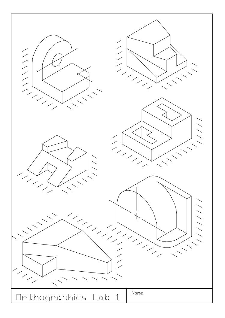
Fill in the missing lines in the following orthographic drawings. Be sure to show all hidden and centerlines.
