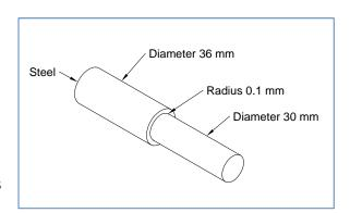
$\begin{array}{lll} \text{Material:} & \text{Steel} \\ \text{Finish:} & \text{Machined} \\ \text{S}_{\text{ut}} : & 600 \text{ MPa} \\ \text{S}_{\text{e}} : & 200 \text{ MPa} \\ \text{K}_{\text{t(bending)}} : & 3.4 \end{array}$
