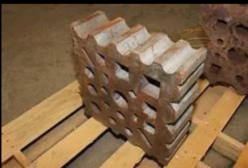
A swage block (or swager block) is a large, heavy block of cast iron or steel used in smithing, with variously-sized holes in its face and usually with forms on the sides. The through-holes are of various shapes and sizes and are used to hold, support or back up a hot bar of metal for further shaping. (wiki)
