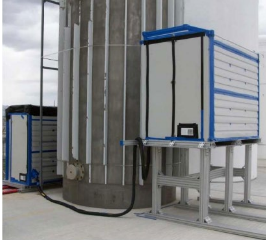
Figure 2: Mini Muon Trackers on either side of a fuel cask during measurement [3].
