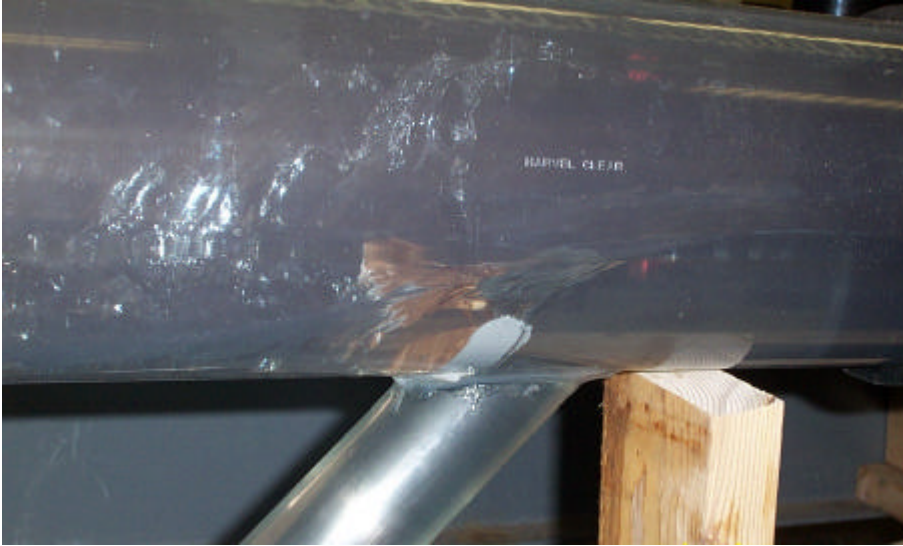
Photo 10. Moderate flow with bottom diversion
