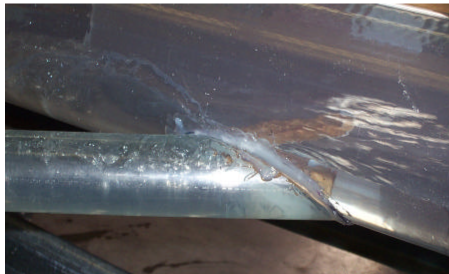
Photo 6. Flow separation in side diversion.
