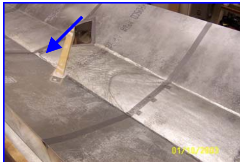
Hydraulic jump location at 2.0 cfs
