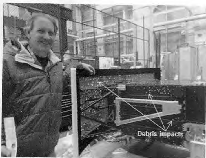
Fig. 6.5 Mark Boslough standing next to the Wide Field and Planetary Camera 2 in 2014 that had been used by the Hubble Space Telescope to take the photos of the Shoemaker-Levy 9 impact shown in Fig. 6.12b. Impact micro-craters on the camera structure have been drilled out, leaving the visible holes (Private collection, M. B. Boslough)
