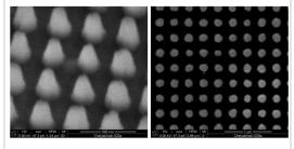
Picture above is SEM images of the plasmonic structure over the photodetectors
