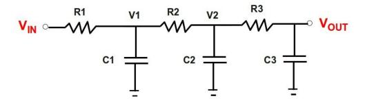
The analysis can be performed by realizing that this is a sequence of voltage dividers. The relation between  $V_{\rm OUT}$  and  $V_2$  is:
