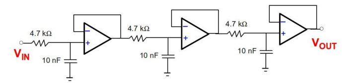
The response (i.e. transfer function) is simply the product of the three individual RC low-pass filters. For three identical sections this is:
