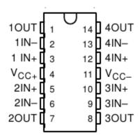
If you choose to use this IC to implement the buffered feedback circuit, you will wire three of the four available op-amps. Connect pin 4 to +15V and pin 11 to -15V. Build only the feedback network shown above using three op-amp buffer stages. Use extreme care here as there are many connections to be made and wiring mistakes can be difficult to track down.
