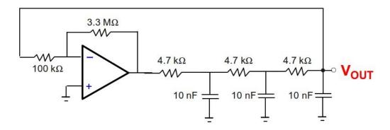
Place the op-amp on the Elvis board (power should be off) so that it straddles a row divider, which allows independent connection of all 8 pins. Connect pin 7 to the +15V and
