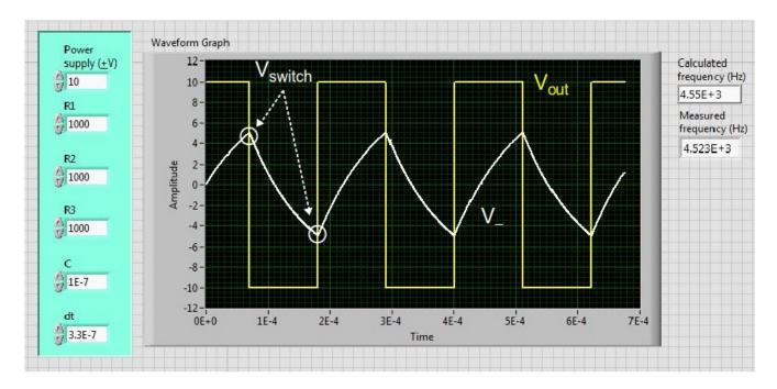
The time (t) in the above equation must be reset to 0 every time the circuit switches. Plot the oscillator output and  $V_-$  on the same Waveform Graph. Note that the VI does not loop; you should generate a pair of waveforms that illustrate oscillator behavior. Measure the frequency of the oscillator output. One option is to use Waveform: Analog Waveform: Measurements: Pulse measurement. Get the period and take its reciprocal.
