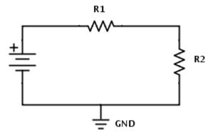
Set the Agilent power supply to 5V DC. If you forgot how to do this, consult the instructions for Lab 1. Use the EZ-hook test leads to connect the power supply output to the circuit. Be sure both red and black leads are connected.
