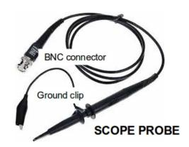
measurement of voltage levels that would otherwise overload the scope input. <u>You must always account for signal attenuation when using a scope probe.</u>
