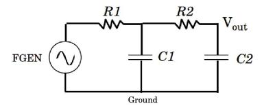
where the second cutoff frequency  $f_c = 1/(2\pi R 2C2)$  should be about an order of magnitude greater than the frequency established by R1C1. Collect amplitude and phase data for this two-pole filter using the BODE analyzer over a suitable range of frequencies. Next, modify the circuit so that R1=R2 and C1=C2. This will establish both poles at the same frequency and thus sharpen the response of the filter. Repeat the BODE measurement and log the data to a file.
