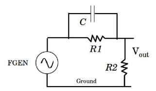
The zero frequency is  $f_{\rm ZERO} = 1/(2\pi R1C)$  and the pole frequency is  $f_{\rm POLE} = 1/[2\pi CR1R2/(R1+R2)]$ . Set R1 = R2 so that  $f_{\rm POLE} = 2f_{\rm ZERO}$  and the amplitude response spans about 6 dB. Record BODE data over an appropriate range of frequencies and LOG data to a removable storage device.
