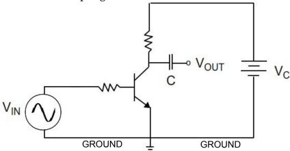
Next set the offset voltage on the function generator to zero and observe what happens. Explain this behavior in the context of the diode experiments done in Lab 6. At this point, show the amplifier results (gain, phase, capacitive coupling, base bias) to the instructor.
