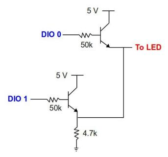
Construct the AND gate shown below and generate the Boolean logic table for all four input combinations.
