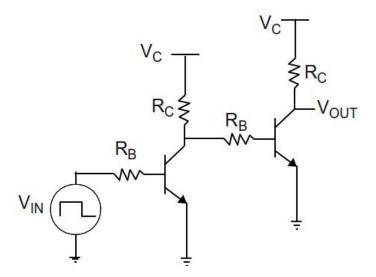
Turn off the Elvis board and add an identical transistor stage to the output of the first transistor as shown in the diagram above. Connect the CH 2 scope probe to the output of the second stage. Power on  $V_C = 5V$  and observe CH 1 and CH 2 on the scope (DC coupling). The second stage should undo the operation of the first, i.e.  $V_{OUT}$  should be the same waveform as  $V_{IN}$ . Two NOT gates in series will restore the input logic.
