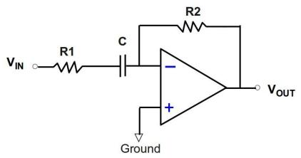
With the same sinusoidal input at frequency 1 kHz, the circuit will differentiate it to produce a 1 kHz cosine wave at V<sub>OUT</sub>, i.e. a waveform that is phase shifted from the input by about 90°.
