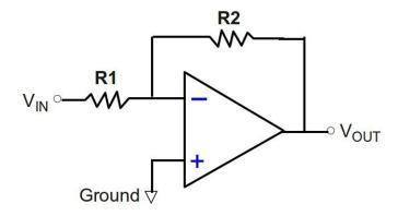
Use R1 = 10 k $\Omega$  and R2 = 50 k $\Omega$ ; neither value is very critical, but always measure components before placing them in the circuit. Be sure to connect the non-inverting op-
