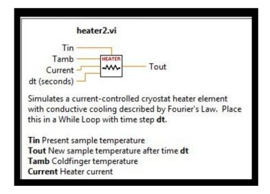
**Tamb** is the reservoir temperature, which is 77K for liquid nitrogen. **Tin** and **Tout** are the input and output temperatures, respectively; wire these to the corresponding terminals of a shift-register. The time  $\mathbf{dt}$  is also the Wait time of the While Loop (note that the subVI requires s not ms).
