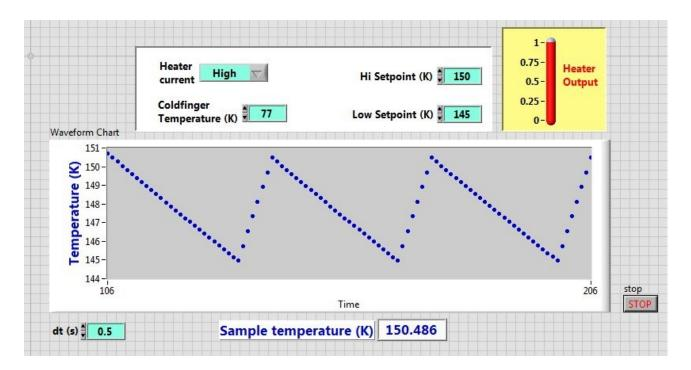
In the next lab, this assigned VI will be interfaced to the Elvis board to control the temperature of a tiny "oven".
