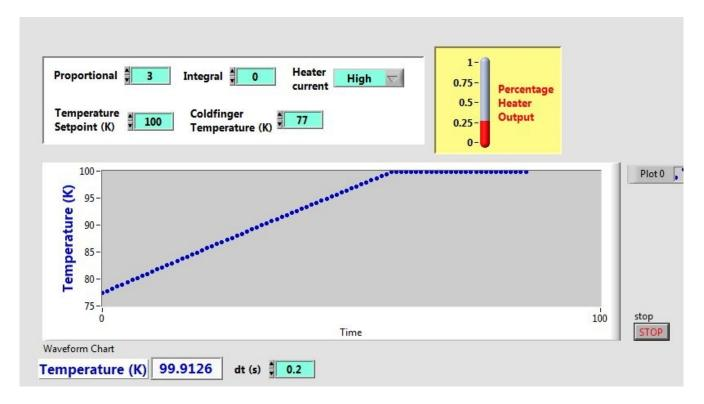
This VI must handle two new issues introduced by the magnitude and phase of the control signal: i) What to do when the amount of current demanded exceeds the capacity of the heater? ii) How to interpret a negative sign on the control signal, i.e. what causes
