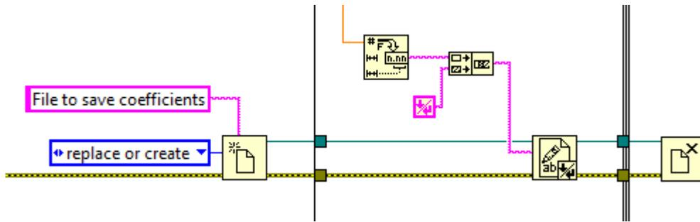
This VI is dealing with two files: one is being read and a second is written. To force the read operation followed by write, connect the **error out** cluster from the File Dialog Express VI to the **error in** terminal of the Open/Replace/Create File VI. Terminate the error cluster in both VIs with a Simple Error Handler.
