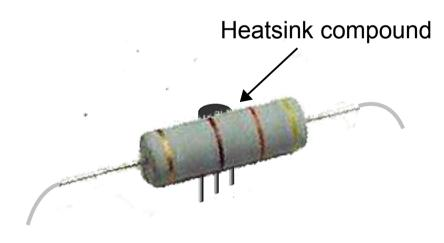
Temperature Sensor: Zener diode based IC
