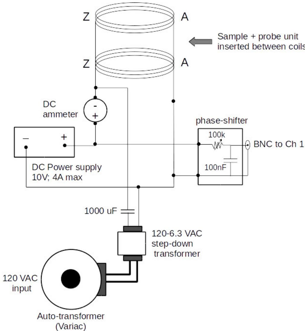
Figure 1: Connect the Helmholtz coils ( $2R = 13.5$  cm) in parallel and separate them by a distance  $R$ . The probe unit (see Figure 2) should fit snugly between the two coils. Set the AC voltage on the secondary winding of the step-down transformer to  $\sim 2$  Vrms. Do not exceed 2A DC into the individual coils, or 4A total.
