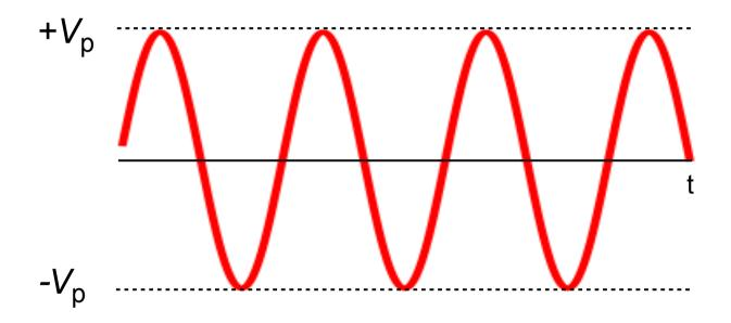
The average voltage of a pure sine wave is identically zero.
