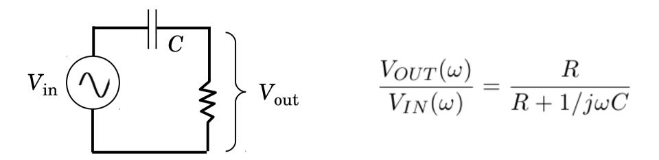
A typical oscilloscope has an *RC* high-pass cutoff in the range 1—10 Hz when AC coupling is used
