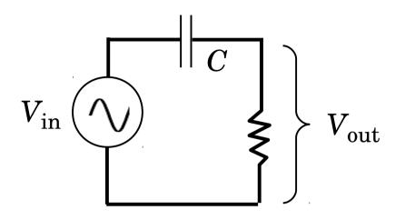
$$\frac{V_{OUT}(\omega)}{V_{IN}(\omega)} = \frac{R}{R + 1/j\omega C}$$
