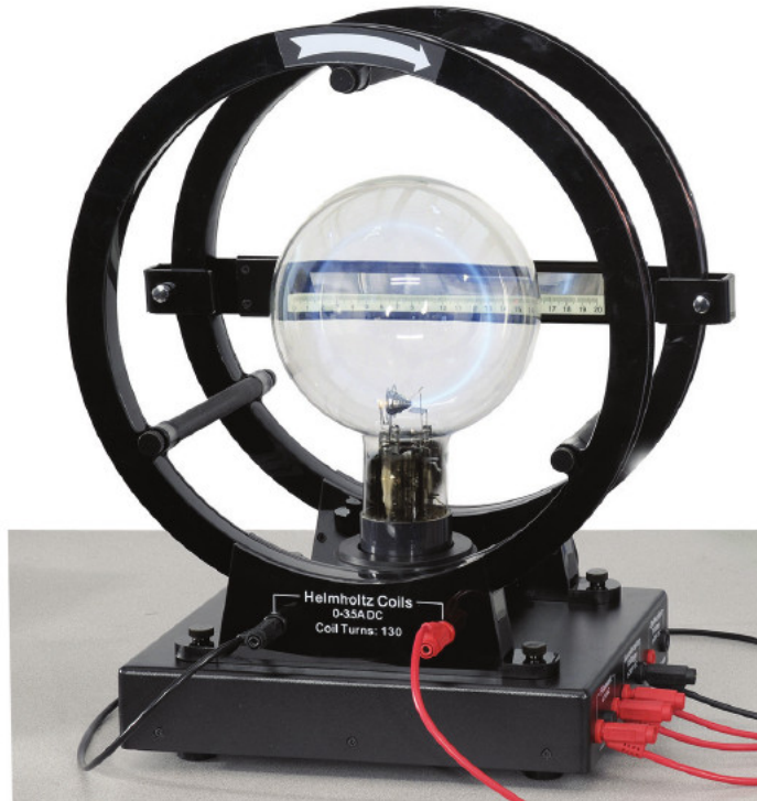
Figure 1: Photo of the e/m measurement apparatus similar to used here. A ruler behind the glass bulb helps measure the electron beam radius ( r ).
