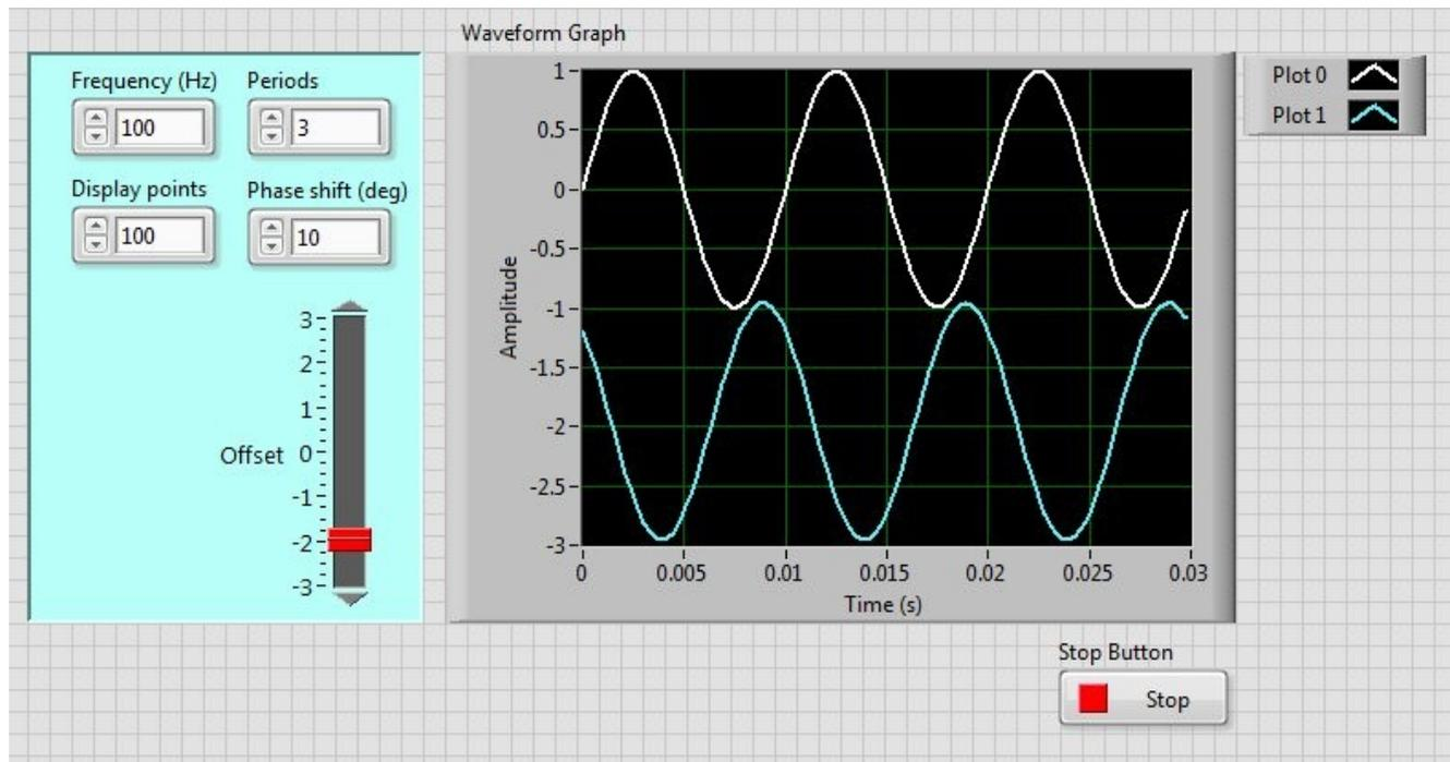
Go to the Block Diagram. The representation of each control must be correct. Display points and periods should be I32. Frequency, phase-shift, and offset are in DBL. Right-click on each icon to access the representation and change as needed.
