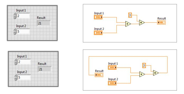
Setting up Block Diagram to flow left-to-right can help visualize logical flow
