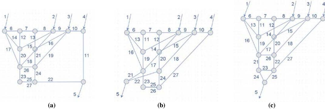
Figure 4. Sub-topologies for VB-links 5-7 from Fig. 3: (a) for VB-link 5, (b) for VB-link 6, (c) for VB-link 7. Notice that on this figure, the VB-links 5, 6, and 7 from Fig. 3 are all labeled as link 5.
