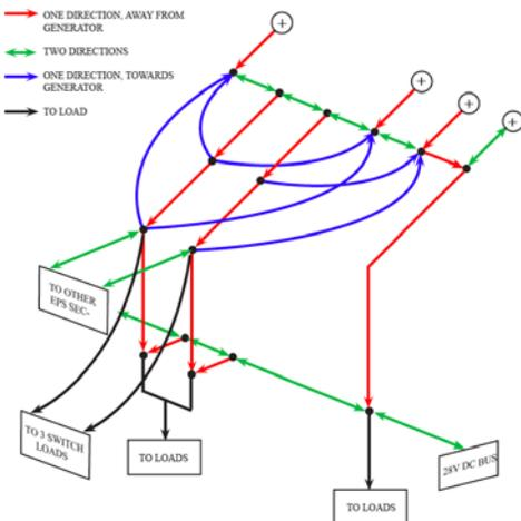
Figure 2. The simplified EPS diagram from Fig. 1 represented using only generators, loads, and links.
