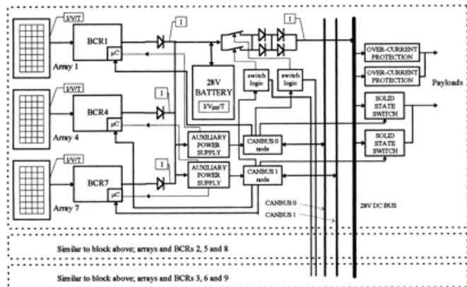
Figure 1. One-third of the UoSAT-12 mini-satellite EPS.<sup>8</sup>
