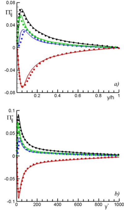
Figure 1.  $\Pi$ -profiles obtained from (3) (solid lines) using DNS data for  $D^{(T)}$  and  $P$ -terms and from DNS (symbols): a) channel flow (Jeyapaul et al., 2014), b) zero-pressure gradient boundary layer over a flat plate (Sillero et al., 2013). Colors: red  $\Pi_{xx}$ , green  $\Pi_{zz}$ , blue  $\Pi_{yy}$ , black  $\Pi_{xy}$ .
