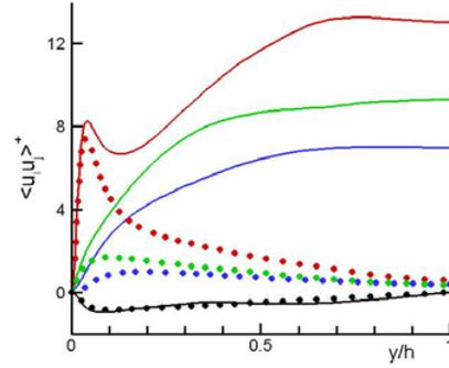
Figure 2. Reynolds stresses obtained using (6). Simulations: solid lines; DNS data: symbols. Colors: red  $\langle u^2 \rangle$ , blue  $\langle v^2 \rangle$ , green  $\langle w^2 \rangle$ , black  $\langle uv \rangle$ .
