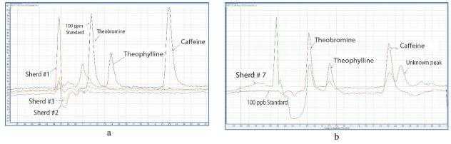
Figure 2. Examples of chromatograms showing analysis results: (a) sherds No. 1, 2, and 3 with no positive cacao residue; and (b) sherd No. 7 with positive cacao residue.
