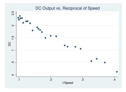
A plot of DC output against one over the wind speed is fairly linear:
