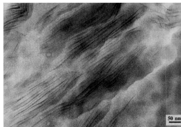
Fig. 7. TEM micrograph of a cross-section of silicate epoxy nanocomposite containing 4 vol. % silicate. From [10].
