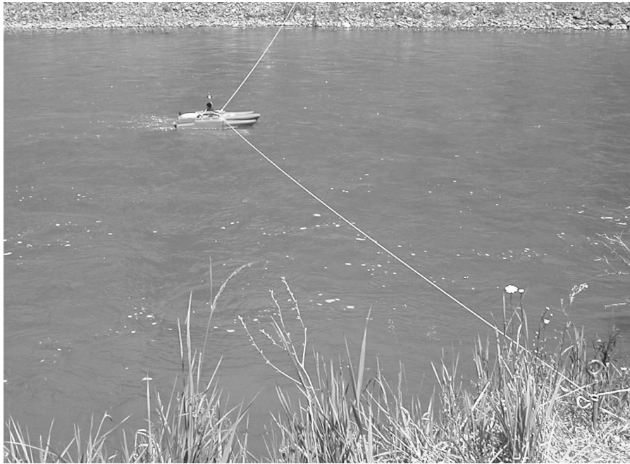
Figure 3 ADCP measurements in the Potlatch River.
