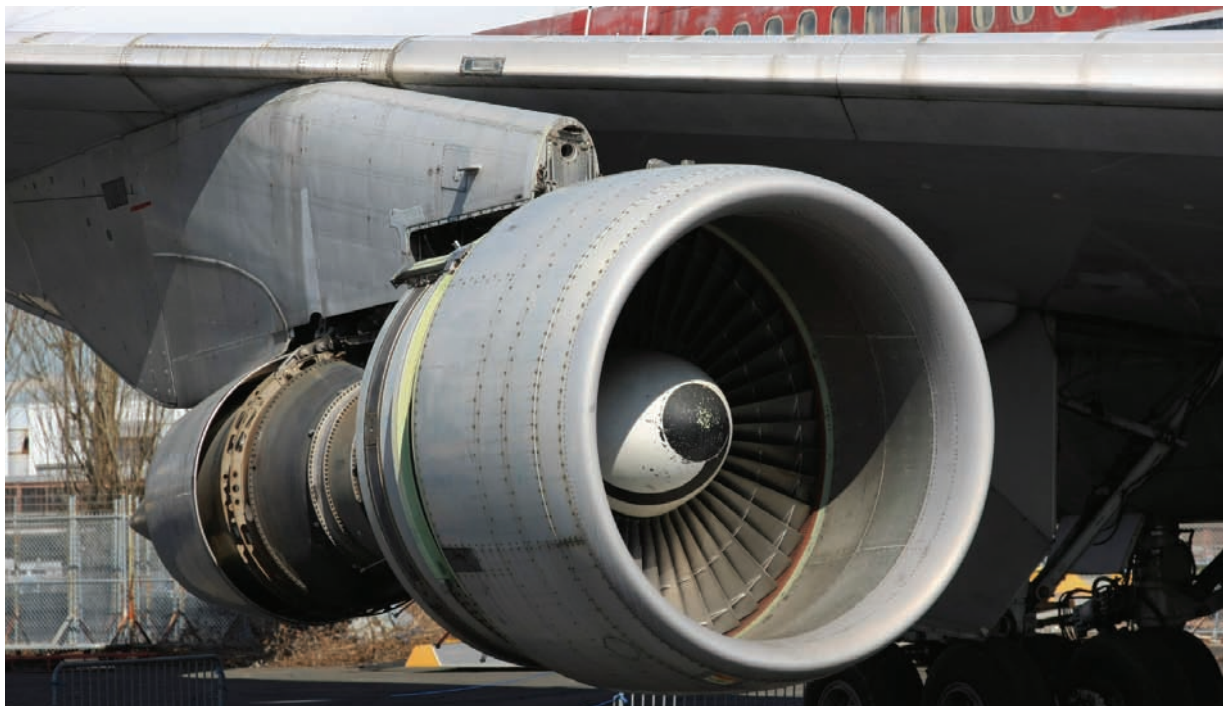
When a plane files through clouds of volcanic ash, the jet engine's heat can melt the ash that flows into it, fusing onto the internal engine parts and causing the engine to lose power and stop.
