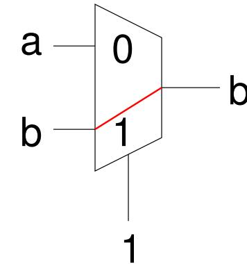
Key idea: The select input wire selects one of the inputs and passes it out to the output.
