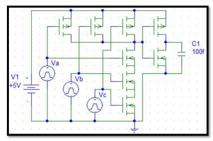
Figure 4. 3-Input AND Logic Gate Circuit
