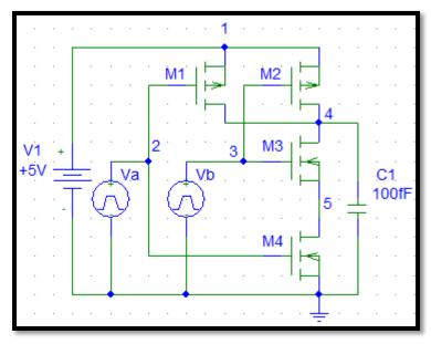
Figure 1. 2-Input NAND Logic Gate Circuit
