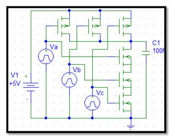
Figure 3. 3-Input NAND Logic Gate Circuit
