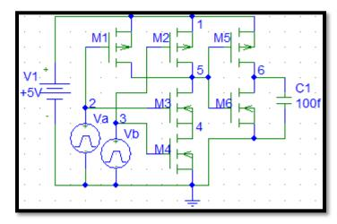
Figure 2. 2-Input AND Logic Gate Circuit
