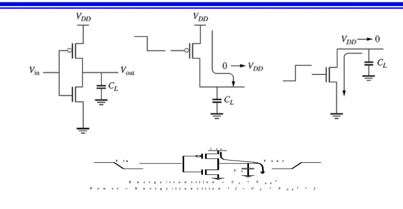
$$P_{d} = \frac{1}{T} \int_{0}^{T} i_{VDD}(t) \cdot V_{DD} dt = \frac{V_{DD}}{T} \int_{0}^{T} C_{L} \frac{dV_{out}}{dt} dt = \frac{C_{L}V_{DD}}{T} \int_{0}^{V_{DD}} dV_{out} = \frac{C_{L}V_{DD}^{2}}{T} = C_{L}V_{DD}^{2} f$$
