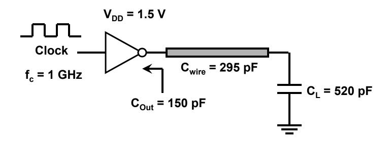
In this circuit, compute the power consumption in the inverter.
