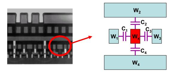
□ If  $W_1$ ,  $W_2$ ,  $W_3$ , and  $W_4$  are grounded (not switching), then the total capacitance that the  $W_x$  wire sees is:
