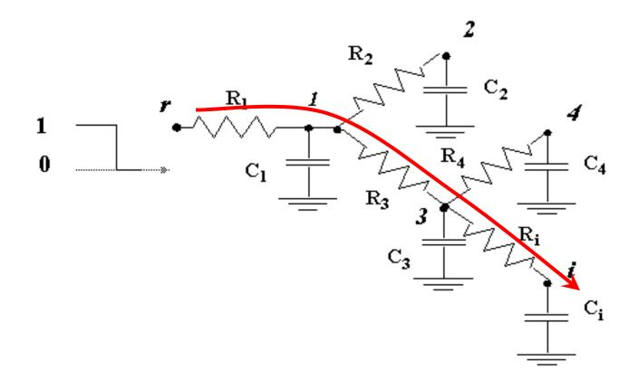
How to compute the delay from node r to node I in this complex RC network?
