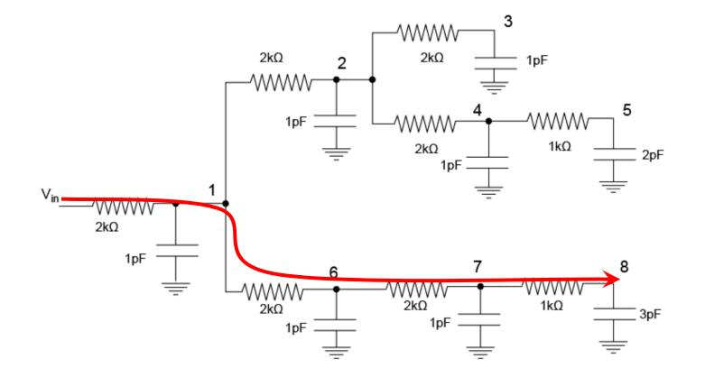
Try this example by yourself. The time constant from Vin to node 8 is 43ns. Therefore, the propagation delay from Vin to node 8 is 30.1 ns
