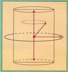
*Rf energy displaces atomic electrons, causing energy to be released on their return to a normal axis*
