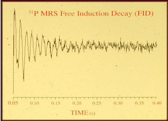
*Energy output from nuclei is acquired, and the frequency of the signal is specific to the atom of interest*
