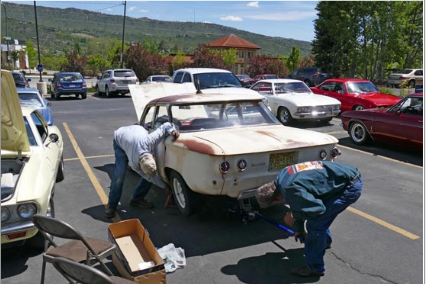
Lube Lubert took out the rear axles and bearings to inspect and re-grease in an effort to find a persistent knocking sound. Actually, the bad bearings survived to get him safely back to Albuquerque on Sunday.
