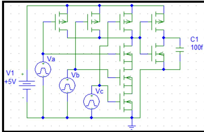
Figure 4. 3-Input AND Logic Gate Circuit
