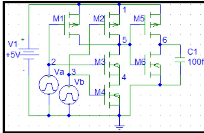
Figure 2. 2-Input AND Logic Gate Circuit
