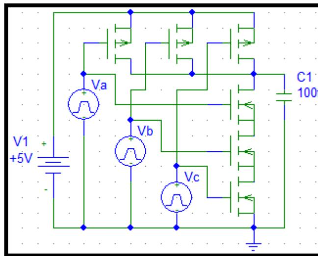
Figure 3. 3-Input NAND Logic Gate Circuit
