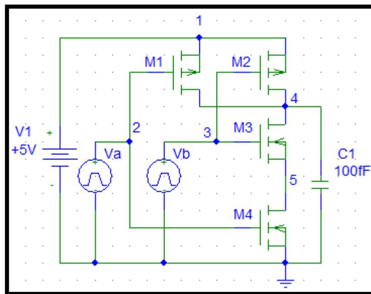
Figure 1. 2-Input NAND Logic Gate Circuit
