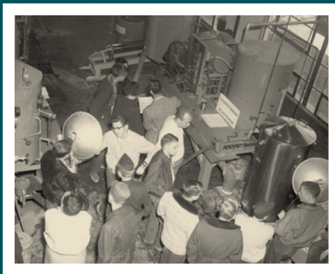
Here students view a Kleinschmidt evaporator, which uses the energy of surface waves in an ocean to manufacture fresh water in a submarine.
